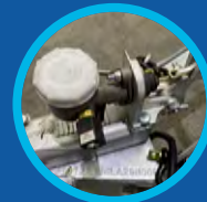
REVERSE SENSOR WITH AUTOMATIC BRAKE RELEASE
