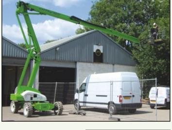
The **HR21 Hybrid AWD** also incorporates **ToughCage** and **SiOPS**<sup>®</sup> technologies. A tough impact resistant composite base and larger cross-section steel give the **ToughCage** strength and durability, while **SiOPS**<sup>®</sup> offers additional operator protection.
