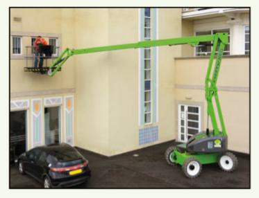
The tough, impact-resistant composite base and larger cross-section steel rails of the HR15's **ToughCage** give extra strength and durability and the multi award winning **SiOPS**® provides additional operator protection.
