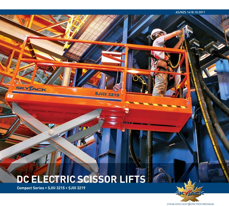
The Compact Series DC Electric Scissor Lifts offer Skyjack's easy to service, low maintenance design in a compact and versatile package. Equipped with variable speed front wheel hydraulic drive, and 90° steering, both models in the Compact Series are capable of maneuvering in the smallest spaces. Featuring a 0.9 m roll out extension deck, these Compact Series models offer work heights up to 7.8 m and 30% gradeability.
