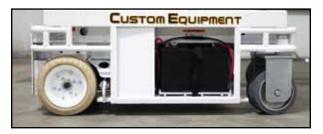
With 360-degree rotating front wheels, and dual rear wheel drive motors, the HB-830's zero turning radius gives the operator a new level of access into the tightest of work spaces. The machine utilizes a highly efficient 24-vdc electrical system, has optional 110v power to the platform, includes secure 4-corner machine tie-down capability, and has a remote emergency down control.
