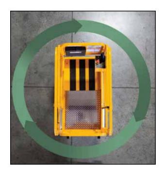
The HB-830 has a 25" by 44.5" work platform and a 19" (CE - 13") slide out.
