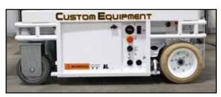
The HB-830 has a long list of standard design features including an integrated battery charger with charge level indicator, decent and tilt alarms, emergency stops, remote raise/lower control station, and a key operated on/off switch. The HB-830 includes fully automatic pot hole protection that meets or exceeds applicable OSHA, ANSI, CE safety standards.
